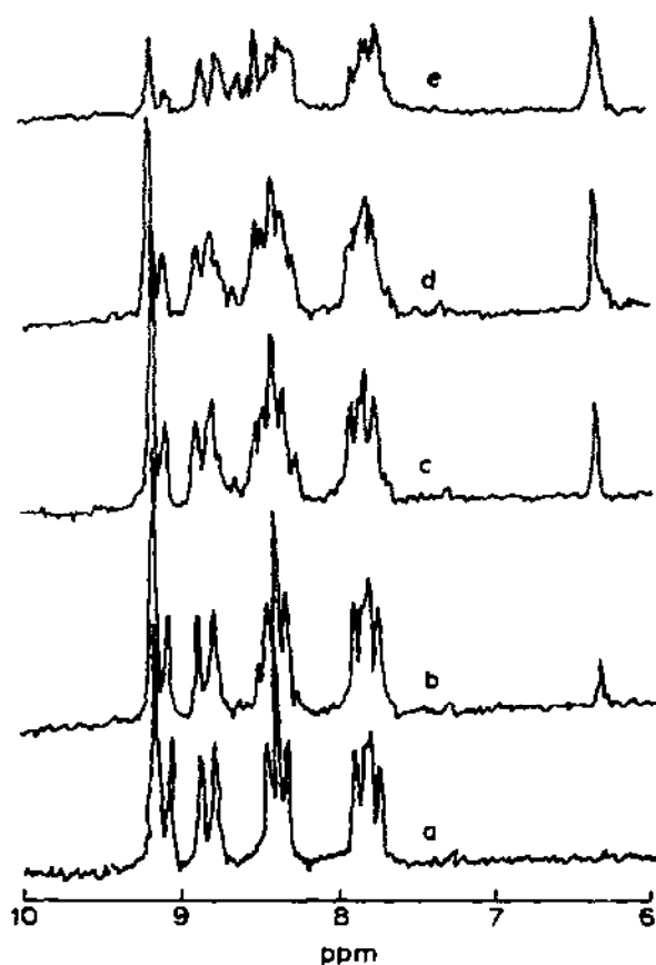
Fig. 22. 90 MHz ^1\text{H} NMR spectra of the reaction of \text{Ru}(5\text{-NO}_2\text{phen})_3^{2+} in \text{CD}_3\text{NO}_2/d_5\text{-pyridine} (5:1, v/v) as a function of time: (a) t = 0 , (b) t = 20 min, (c) t = 55 min, (d) t = 115 min, (e) t = 400 min; temperature = 35^\circ\text{C} . For (e) the spectral amplitude is 1/2 \times . Reprinted with permission from ref. 153.
