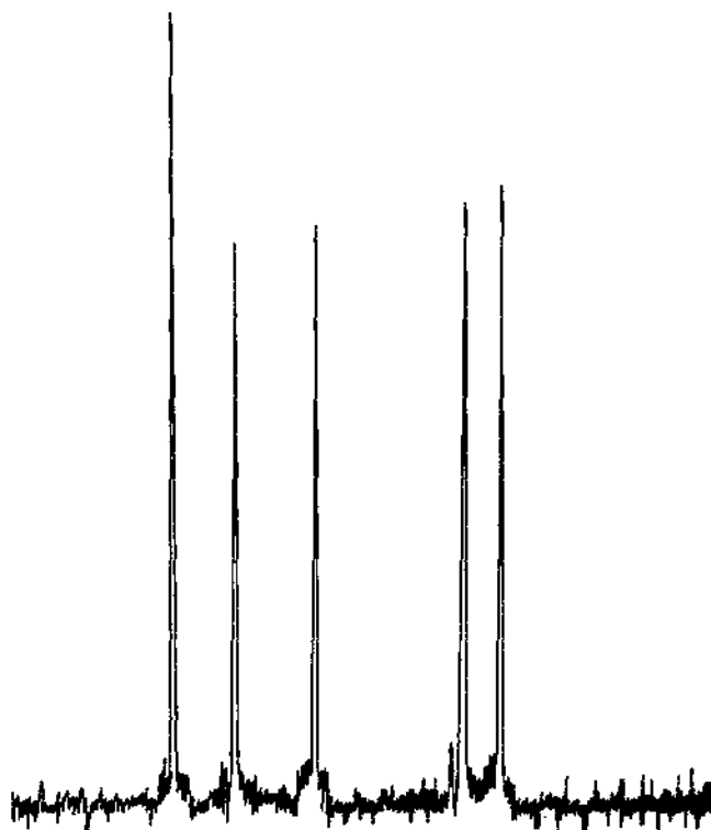
Fig. 27. ^{13}\text{C} NMR spectrum of [\text{Ir}(\text{bpy})_3](\text{NO}_3)_3 in \text{H}_2\text{O}-\text{D}_2\text{O} . Chemical shifts starting at left are: -89.46 , -83.77 , -76.69 , -63.34 , -60.04 ppm relative to internal dioxane standard. No additional peaks occur above the noise level from -110 to +90 ppm. Reprinted with permission from ref. 222.
